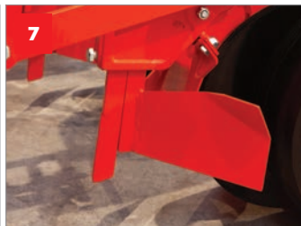
7 CLOD REMOVER The adjustable clod remover cleans dry soil and clods in front of the row units.
