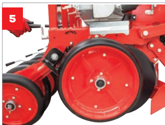
5 DEPTH ADJUSTMENT Depth adjustment from 1 to 10 cm due to rubber gauge wheels allows to seed precisely on uneven field conditions.
