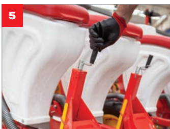
5 DEPTH ADJUSTMENT Working depth adjustment is possible from 1 to 10 cm from the wheel adjuster.
