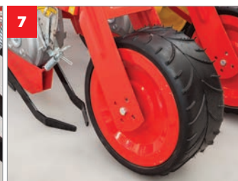
7 REAR PRESS WHEEL 500X175 rubber press wheel is standart on coulters type row units.
