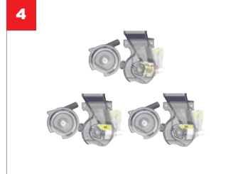
4 SEED FLOW PLATES According to seed type , there are three types of seed flow plates prevent seed breaks because of seed overloading on seed meter. C1 : Maize, Sugarbeet, Soya e.t.c. C2 : Small Size sunflower C3 : Big size sunflower and pumpkin
