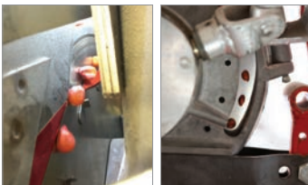
For perfect singulation for all kind of seeds on all row units ,selectors can be adjusted from the outside of the distributor by a metering scale.
